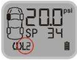
Function: The system will issue a Low Pressure Level 2 Alarm when the tire pressure is 25% lower than the standard.
