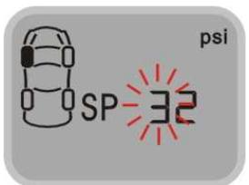
Press the E key to access this program. The first number of the Standard Pressure of the Front Left tire is flashing, as shown in
