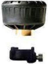
First connect the meshing parts of the Lock and the Transmitter to make them an integrated part, then screw the Transmitter together with the Lock firmly onto the valve, as shown in the left figure.
