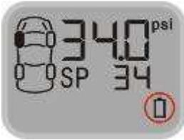
Function: The system will issue a warning alarm when the battery power is not enough to afford the Monitor to work when the Monitor powered by the battery group.
