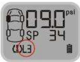
Function: The system will issue a Low Pressure Level 3 Alarm when the tire pressure is 50% lower than the standard.
