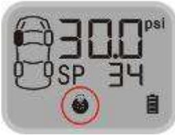
Function: The system will issue a Quick Leaking Alert when the pressure drop exceeds 2.8psi within 12 seconds.
