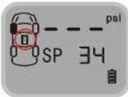
Function: If one Transmitter fails to work, or the Monitor can't receive the data because of the RF interference for a certain time, the system will issue a Transmitter Trouble Alarm.
