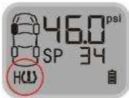
Function: The system will issue a High Pressure Alarm when the tire pressure is 25% higher than the standard.
