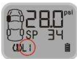
Function: The system will issue a Low Pressure Level 1 Alarm when the tire pressure is 12.5% lower than the standard.
