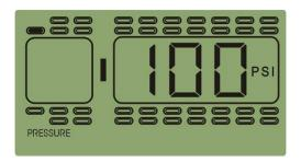
3. Then press S for 3 seconds to set the first digit which flashes. Press up or down arrow key to adjust the value to 1.
