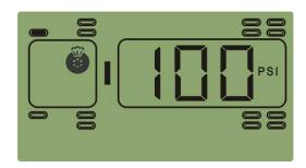
Function: the system will issue a quick leak alarm when the pressure drops more than 2.8 psi within 12 seconds.
