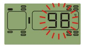
Function: When the temperature around the transmitter equals or exceeds  $90^{\circ}\text{C}$ , the system will issue the high temperature alarm.
