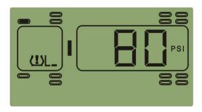
Function: the system will issue low pressure level 1 alarm when the tire pressure is 12.5% lower than the standard.
