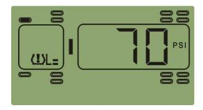
Function: the system will issue low pressure level 2 alarm when the tire pressure is 25% lower than the standard.
