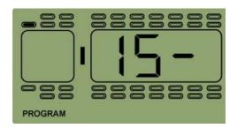
5. Press again to program the third digit which flashes. Press up or down arrow key to adjust the value.
