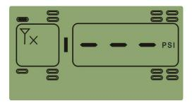
Function: If one transmitter fails to work, or the monitor cannot receive the data because of the RF interference for 20 minutes, the system will issue a transmitter trouble alarm.
