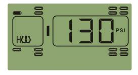
Function: the system will issue the high pressure alarm when the tire pressure is 25% higher than the standard.
