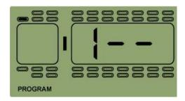
4. Once finish programming of the first digit, press  $\longrightarrow$  to start programming the second digit which flashes. Press up or down arrow key to adjust the number.
