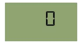
2. Under alarm record inquiry interface, Press → key to check through the record. If there is no operation within 3 seconds, it will automatically display the record data (pressure, temperature and time) in turn, each data displays 3 seconds.
