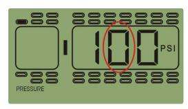
5. Once finished programming the second number, press → to program the third digit which flashes and then press up or down arrow key to adjust the value to 5. Then press S for 3 seconds to save the setting.
