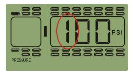
4. Once finished programming the first number, press → to program the second digit which flashes and then press up or down arrow key to adjust the value to 0.
