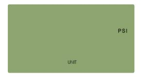
2. Under any interface displaying temperature or pressure, press S key for 3 seconds to start programming. Take change the temperature unit as an example: under the temperature unit interface, press S key for 3 seconds, the temperature unit "C" starts flashing. Press up or down arrow key to select the needed temperature unit.
