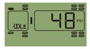
Function: the system will issue low pressure level 3 alarm when the tire pressure is 50% lower than the standard.
