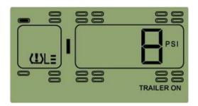
Function: the system will issue low pressure level 3 alarm when the tire
