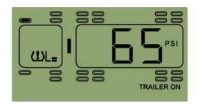
Function: the system will issue low pressure level 2 alarm when the tire pressure is 25% lower than the standard.
