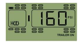
Function: the system will issue the high pressure alarm when the tire
