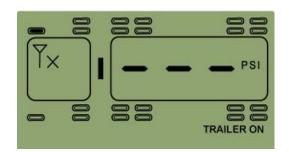
Function: If one transmitter fails to work, or the monitor cannot receive the data because of the RF interference for 20 minutes, the system will issue a transmitter trouble alarm.
